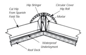
Figure 8.5 Hip Section Showing Circular Cover Hip
