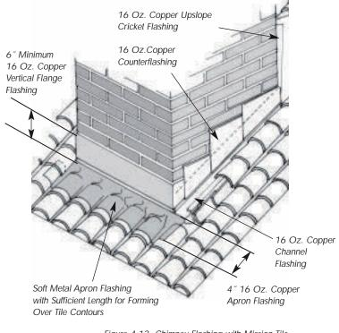
Figure 4.13 Chimney Flashing with Mission Tile
