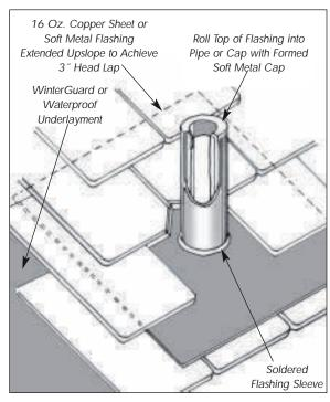
Figure 4.16 Pipe Penetration Flashing for Shingle Tile
