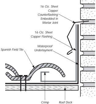
Figure 8.11 Section Showing Flashing Under Side of Tiles
