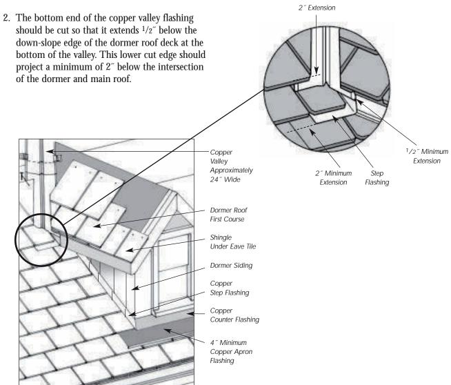
Figure 4.11 Open Valley at Main Roof to Dormer Juncture with Flat Shingle Tile
