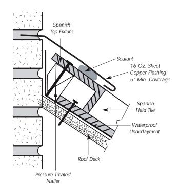
Figure 8.12 Deck Section Showing Flashing Over Top of Tiles
