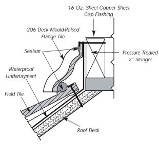
Figure 7.8 Deck Section Showing 206 Deck Mould-Raised Flange Tile
