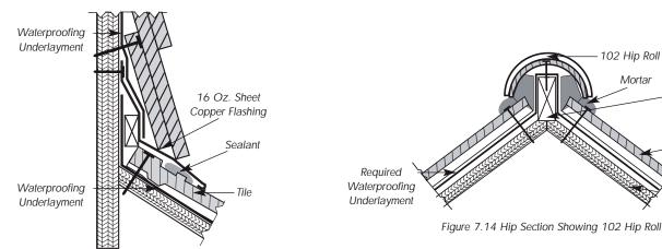
Figure 7.13 Section Showing Flashing Under <sup>3</sup>/8" Flat Shingle Tiles
