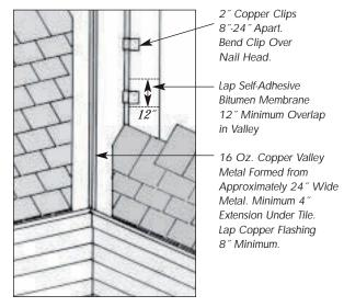
Figure 4.4 Typical Open Valley Flashing for Shingle Tile
