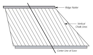
Figure 3.6 Chalking Vertical Lines to Guide Installation
