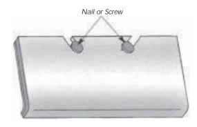
Figure 3.11 Ridge and/or Under Eave Course Notched and Fastened
