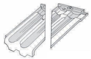
Figure 7.4 Cut Hip - Left and Cut Valley - Right
