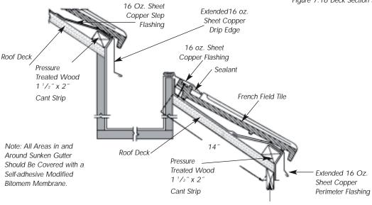
Vertical Fascia Figure 7.17 Section Showing Sunken Gutter Treatment
