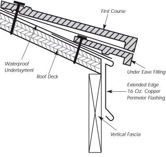
Figure 3.9 Under Eave Fitting for Starter Course Example of Interlocking Tile
