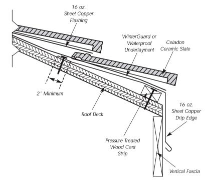
Figure 4.7 Section of a Closed Valley
