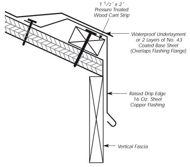
Figure 7.2 1 1/2" x 2" Cant Strip Installed Directly to the Wood Deck
