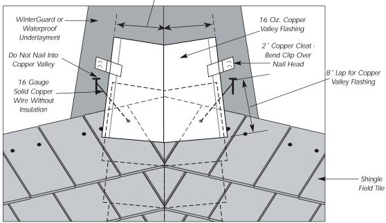
Figure 4.8 Typical Closed Mitered Valley for Flat Shingle Tile with Stepped Flashing
