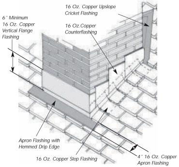
Figure 4.12 Chimney Flashing with Shingle Tile
