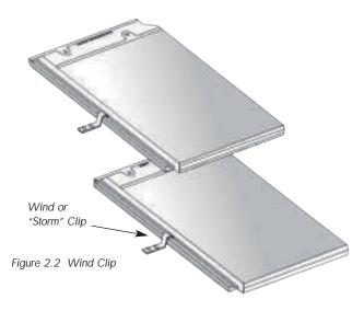
Note: In high wind regions, install each tile with #8 or #9 brass flathead phillips or square drive screws and/or use wind clips. Wind clips and sealants may be required by the local building codes.
