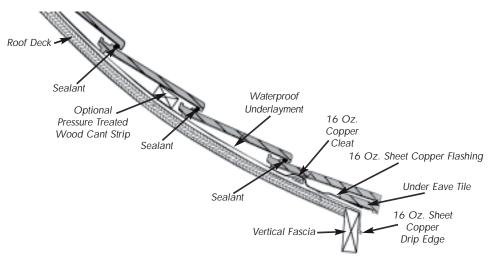
Figure 4.20 Flashing to Curved Rafter (for Interlocking Tile)
