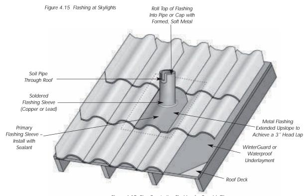
Figure 4.17 Pipe Penetration Flashing for Spanish Tiles
