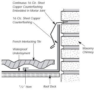
Figure 7.11 Section Showing Flashing Under Side of Tiles
