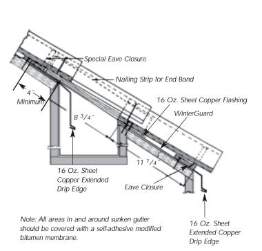
Figure 8.7 Section Showing End Band Over Concealed Gutter For  $13^{1}/4^{\circ}$  Spanish Tile
