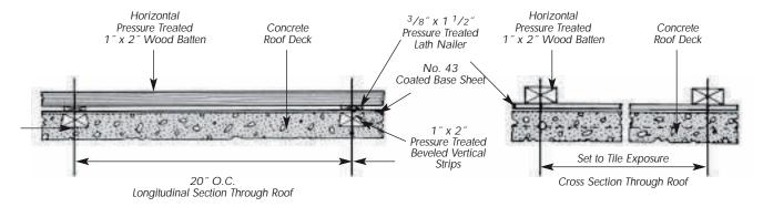
Figure 7.12 Application of Batten System to Poured Concrete Roof Deck
