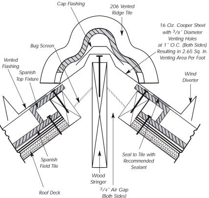
Figure 8.1 206 Vented Ridge Tile Detail
