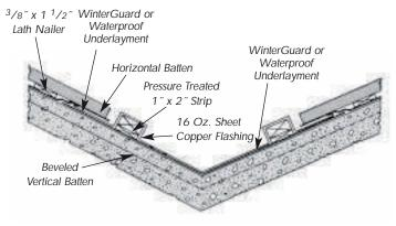
Figure 7.9 Section Showing Valley Flashing on Poured Concrete Roof Deck
