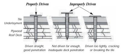
Figure 2.1 Proper Nailing Techniques for Plywood Deck
