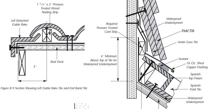
Figure 8.10 Section Showing Flashing Under Spanish Tiles
