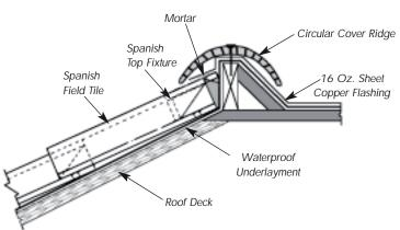
Figure 8.3 Deck Section Showing Circular Cover Ridge
