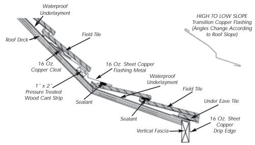
Figure 4.19 Flashing at Low Slope to High Slope (for Interlocking Tile)
