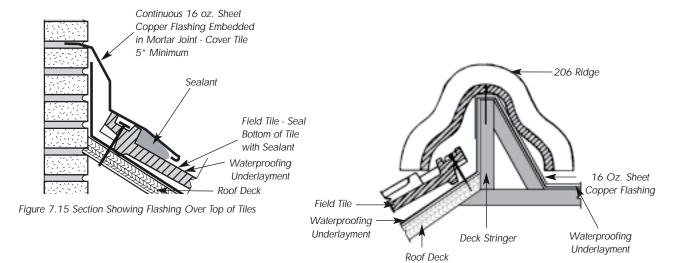
Figure 7.16 Deck Section Showing 206 Ridge
