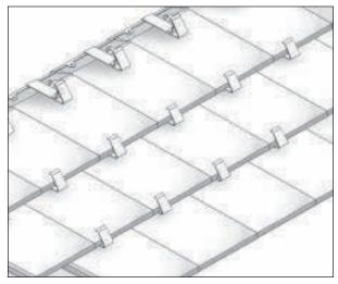
Figure 2.3 Recommended Snowguard Spacing
