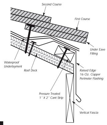
Figure 3.8 Cant Strip for Starter Course Example of Flat Shingle Tile
