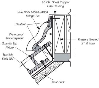
Figure 8.8 Deck Section Showing 206 Cut-Off Ridge
