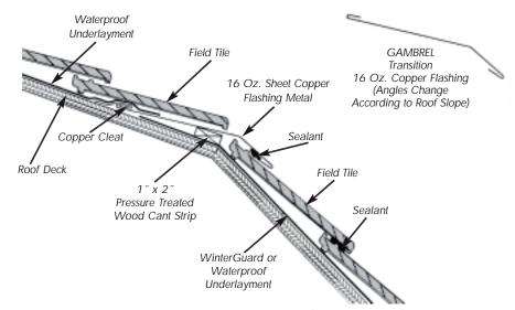
Figure 4.18 Flashing at High Slope to Low Slope (for Interlocking Tile)
