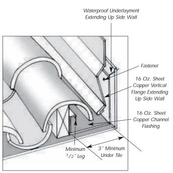
Figure 4.10 Channel Flashing with Pan and Cover Tile
