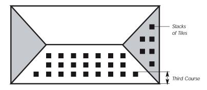
Figure 3.10 Distribution of Tile Over Roof
