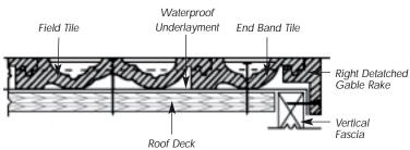
Figure 7.10 Section Showing Right Gable Rake and End Band
