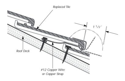
Figure 12.2 Replacement Detail
