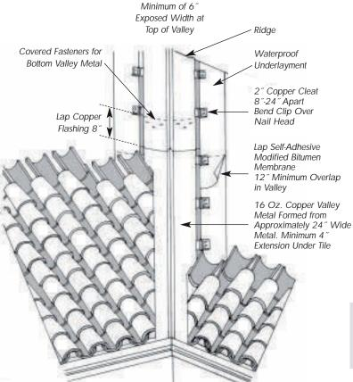
Figure 4.3 Typical Open Valley Flashing for Pan and Cover Tiles
