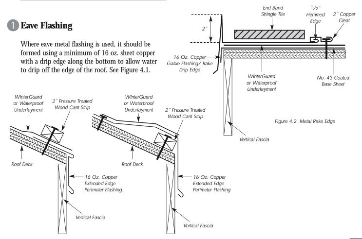
Figure 4.1 Perimeter Flashing with Cant Strips
