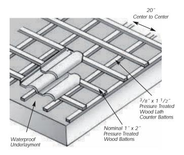
Figure 3.3 Batten System of Attachment for Concrete Deck
