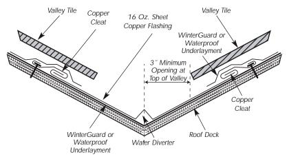
Figure 7.7 Cross Section Showing Valley Flashing on Wood Roof Base
